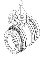
Wrong methods for Hoisting Ball Valve
